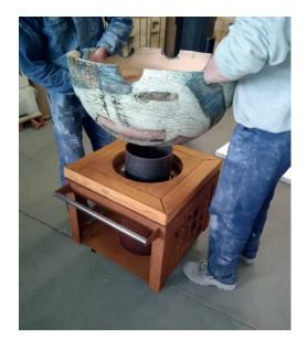
Place the steel cone inside the ceramic bowl and screw the three screws you removed before.
